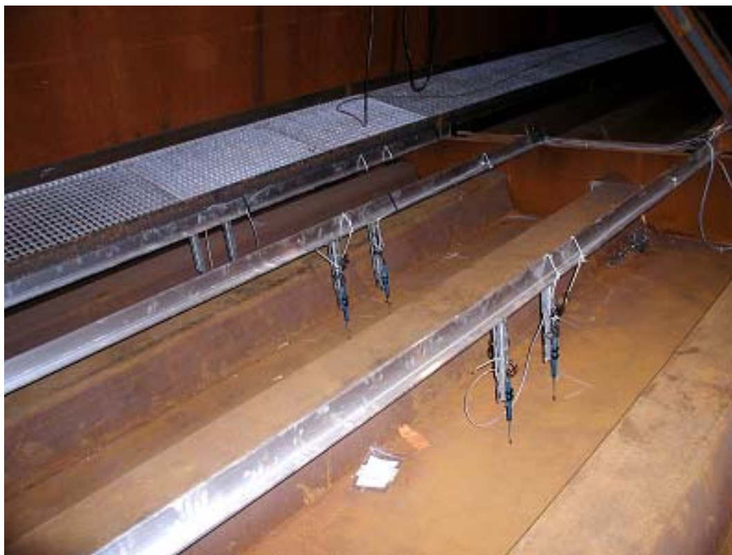
Photo 16: Checking "patch-loading" during a launch
