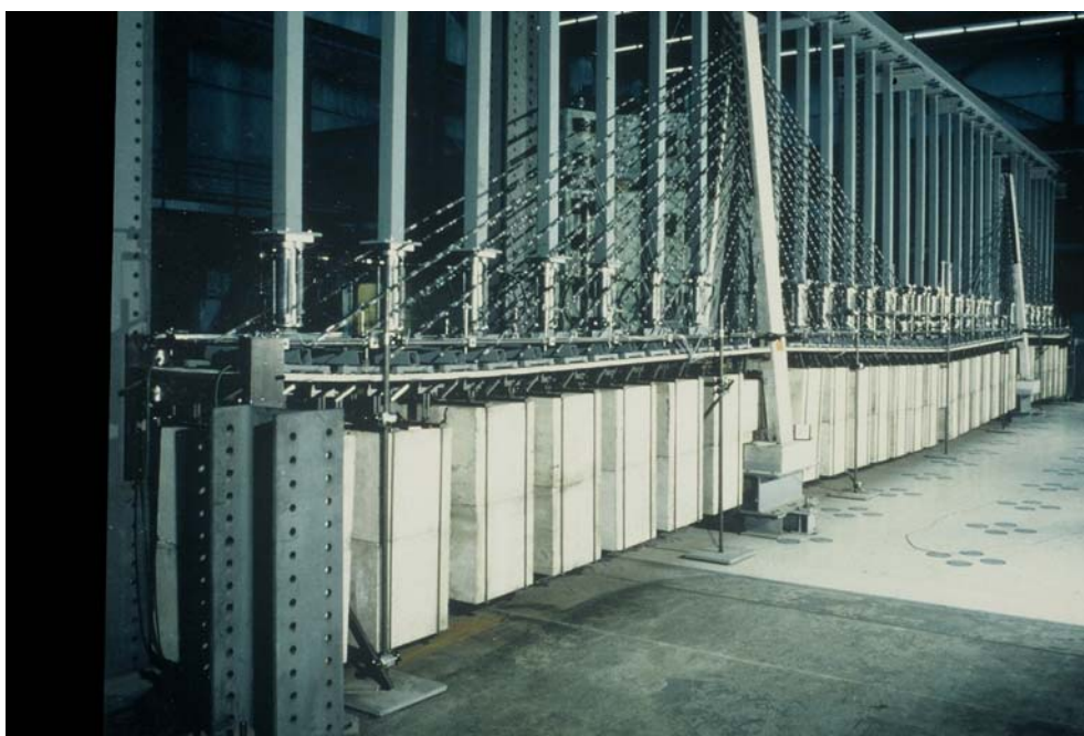
fig. 5: Tests on cable-stayed bridge with slender concrete deck
