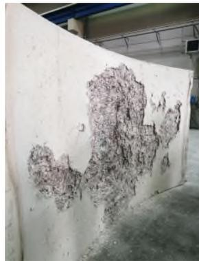
**FIGURE 5 VOUSOIRS FIBRE APRES ESSAI AU FEU**
