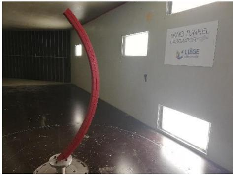
Figure 2. aeroelastic model in wind tunnel
