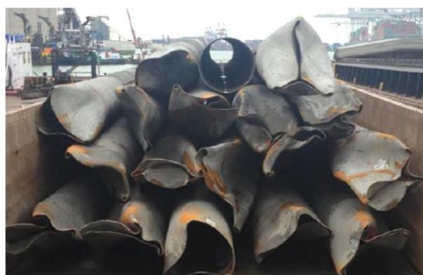
Figure 2. Pile toe failure Amazonehaven [2]
