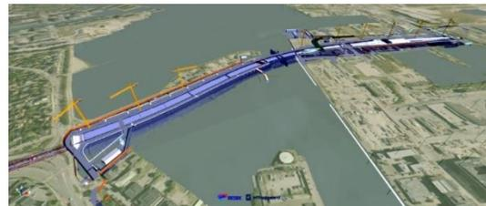
Figure 1: 4D model of the Nordhavn tunnel with temporary structures
